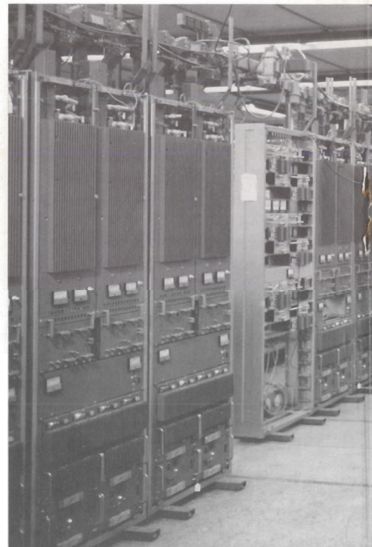
HP network analyzer anchors final testing of microwave radio systems produced for national and international markets by Telettra near Milan.
