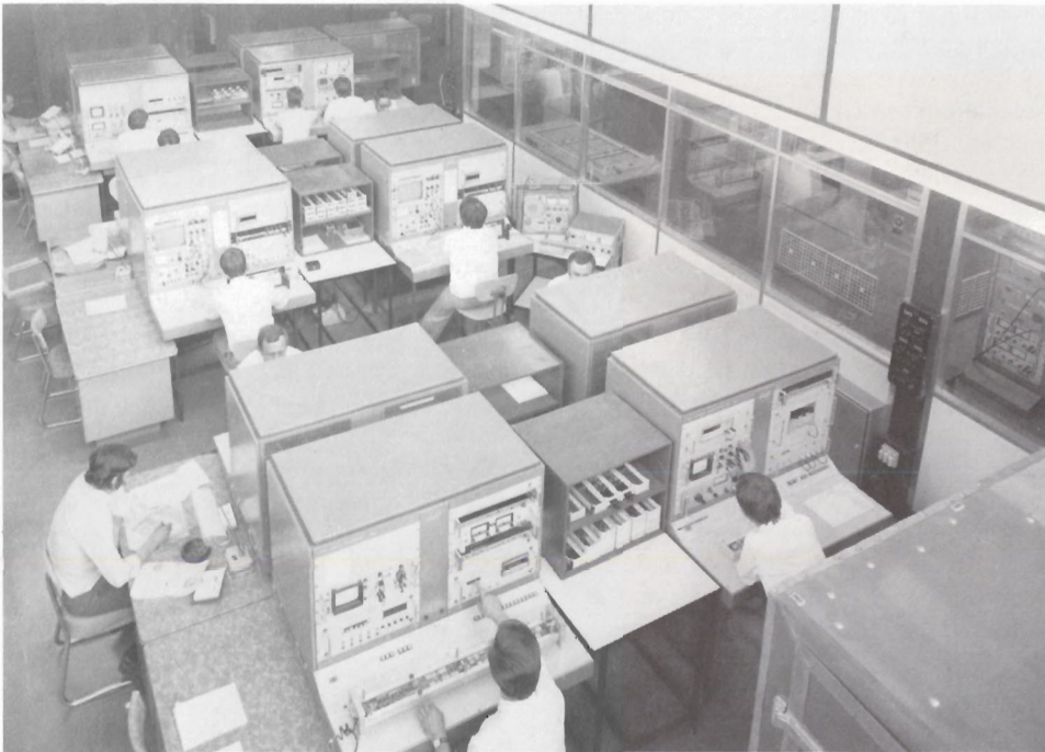
Highly sophisticated electronic test equipment is used by Electronic Marcel Dassault in Paris to test aircraft transponder units.
